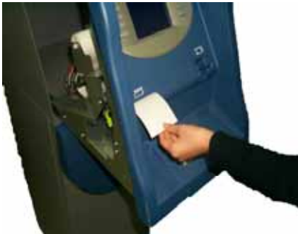
Fig 5.5a Loading the Receipt Paper
